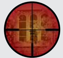
Low Battery indication as viewed through the dayscope
